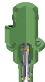
Direct Drive Section View
