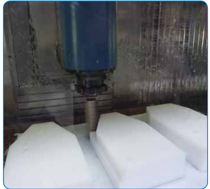
Almatec’s E-Series Plastic AODD pumps are machined from solid plastic blocks of polyethylene (PE) or polytetrafluoroethylene (PTFE), allowing the pumps to handle the harshest environments.
