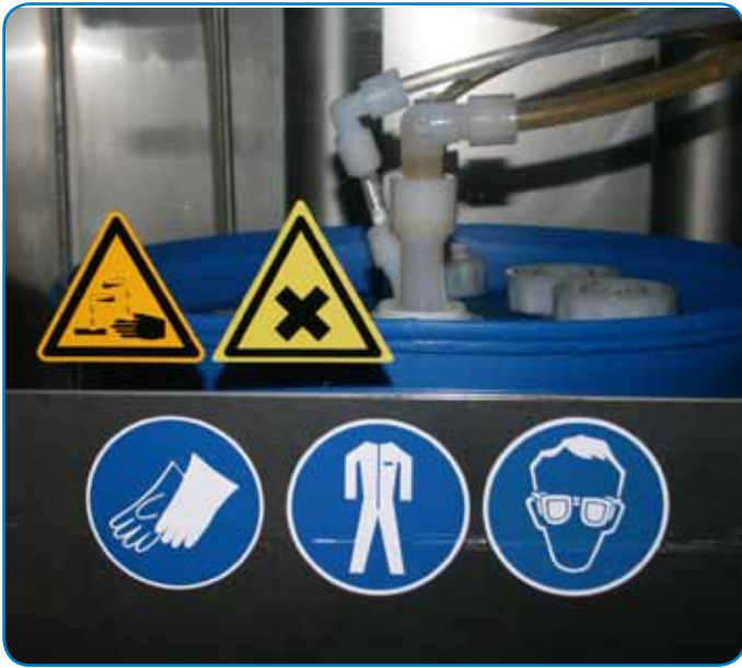
Personal Protective Equipment (PPE) symbols indicate what must be worn when handling a particular hazardous material, including hand protection, protective clothing and glasses.
