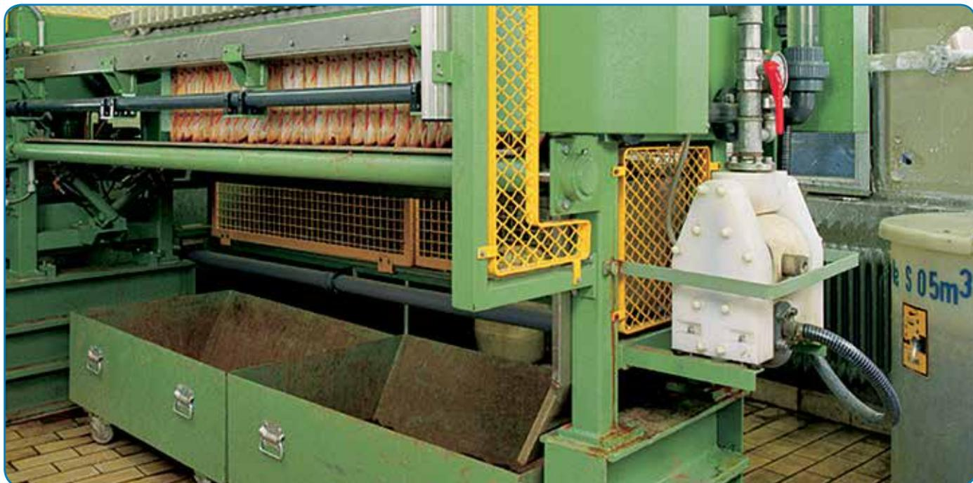
Filter presses take a slurry that contains both solids and liquids and uses a series of filters to “dewater” the mixture so that slurry “cakes” are formed while the remaining liquids are filtered out. AH Series AODD Pumps from Almatec® are a popular choice in filter-press systems because they offer reliable high-pressure operation and product containment while being compatible with the many abrasive or corrosive fluids and chemicals that are a staple of the process.
